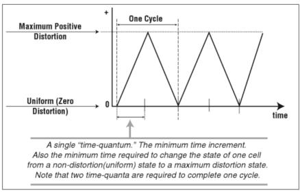
Figure 2.2: Linear unipolar oscillation (sawtooth)
