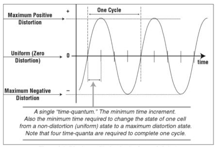
Figure 2.3: Bipolar oscillation in the form of sin(ωt)
